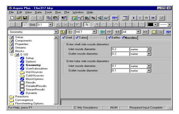
Shell inlet nozzle diameter—specify the diameter of the shell inlet nozzle; refer to reference two for the diameter; if literature values are unavailable, a good starting value is one fourth the shell diameter for liquid flow and half the shell diameter for vapor flow Shell outlet nozzle diameter—specify the diameter of the shell outlet nozzle; this value should be the same as the inlet diameter when there is not a phase change
