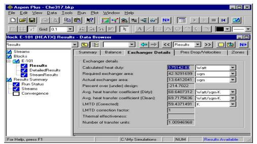
well below the required area. You can also notice the calculated heat transfer coefficient. Aspen calculated a value of 68.6 W/m<sup>2</sup> K, which is below the estimated value of 150 W/m<sup>2</sup> K. The results show that more area is needed for heat transfer and the heat transfer coefficients need to be increased. However, before changing the geometry of the exchanger, you need to check the rest of the result pages, starting with the pressure drop.
