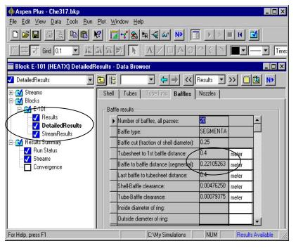
As said before, Aspen calculated the baffle spacing. (BS = 0.22 meters) Detailed Results also show results for the shell, tubes, and nozzles.
