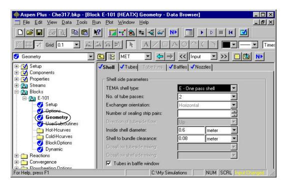
Now begin the layout by clicking on the geometry subfolder at the left-hand side of the screen. The screen above is the input page for the shell dimensions. Enter in the appropriate information.
