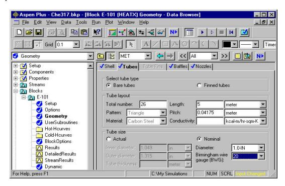
**Select tube type**—either bare or finned type tubes; *generally, bare tubes are used* **Total number**—specify the total number of tubes
