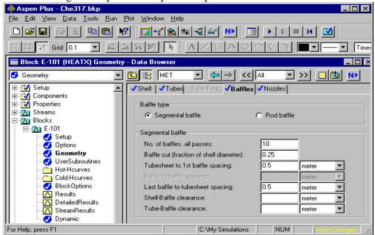
**Baffle type**—choose either segmental baffle or rod baffle; segmental baffles are typical 'wall' baffles while rod type are simply rods that cause more turbulent flow within the shell; each baffle type has a separate input sheet (the segmental baffle input is shown above); examples of baffle types can be seen on page 11-42 of Perry's 7<sup>th</sup> edition.
