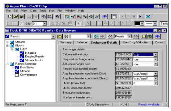
More results for the exchanger can be seen under the "Detailed Results" section under the Results page. Shown below is the baffle results page.
