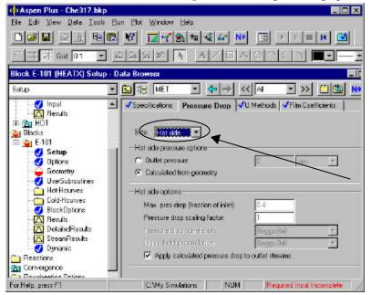
appear. Here, you need to specify how Aspen will calculate the pressure drop of the heat exchanger. We will have Aspen calculate pressure drop from the geometry of the heat exchanger. This option is shown at left and is the preferred option.
