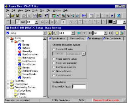
The input page for the overall heat transfer coefficient appears next. (Shown at left) You need to specify how Aspen will calculate the U-value for the exchanger. There are several options explained below. For this example, the U-value will be calculated from "|Film coefficients."
