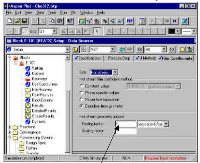
The input page is shown at left. Here is where you need to specify how Aspen will calculate the individual heat transfer coefficients. (Note\*: This page only needs to be filled out if the U-value is calculated from "Film coefficients".) This page is very similar to the **U methods** input page and fortunately the calculation options are the same. The example will use the "Calculate from geometry" option.
