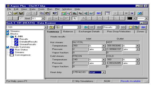
Now check the **Exchanger Details** page (shown below). Make sure to look at the required exchanger area and the actual exchanger area. As you can see, the actual area is
